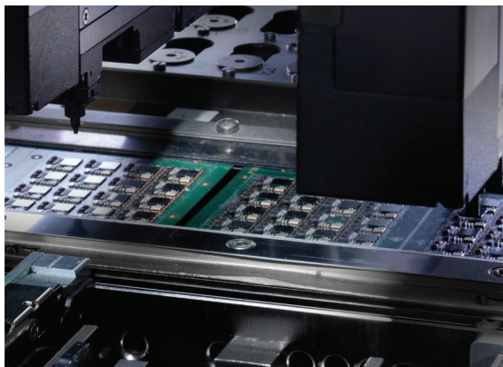
K&S and shows a device attach taking place
